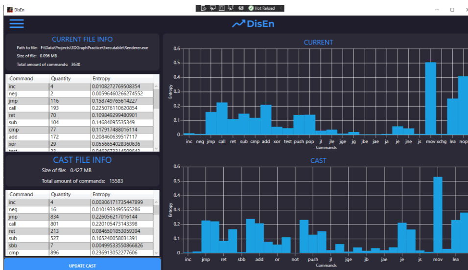
Fig. 1 – Example of disassembling two files and how they differ from each other
